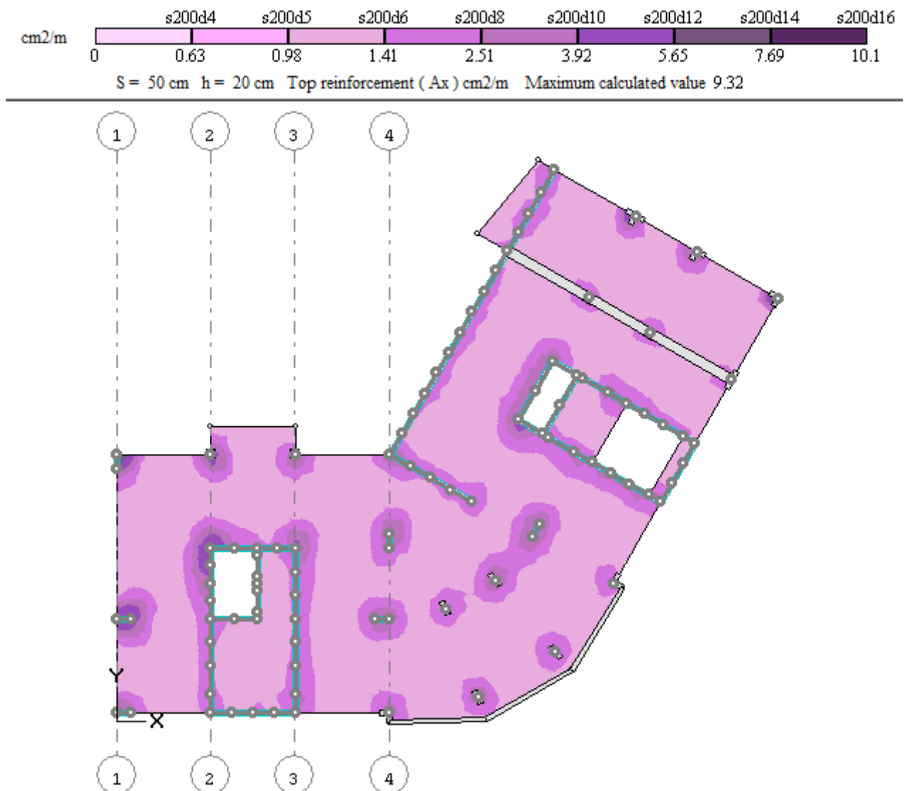
Figure 2.4.9 Contour plot of reinforcement Ax along the upper edge of the slab
